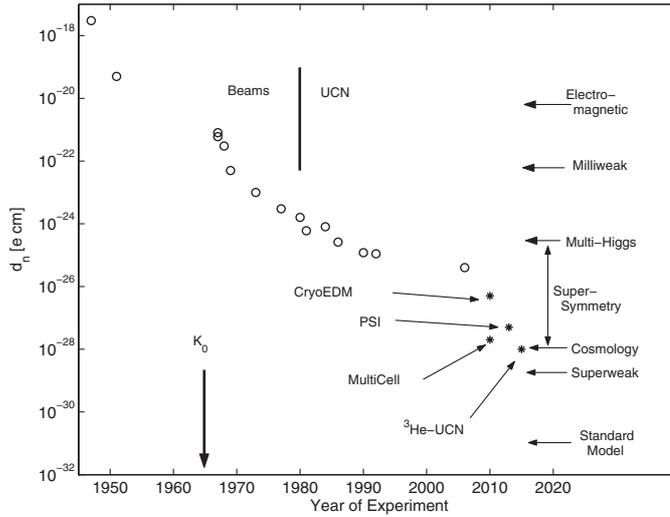
**Figure 1.** History of the sensitivity of neutron EDM searches, compared with some theoretical suggestions as to the magnitude. The use of stored ultracold neutrons (UCN) eliminated the motional magnetic field effect that was a limiting systematic for neutron beam experiments, as described in the text. The points marked with \* are the anticipated limits from experiments presently under development or proposed, and will be discussed in this paper.
