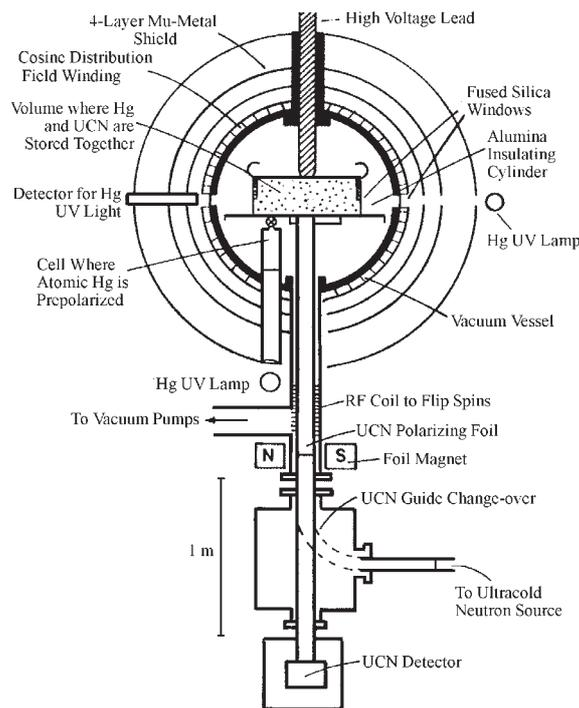
Figure 7. Schematic of the ILL UCN EDM experiment incorporating a  $^{199}\text{Hg}$  comagnetometer.
