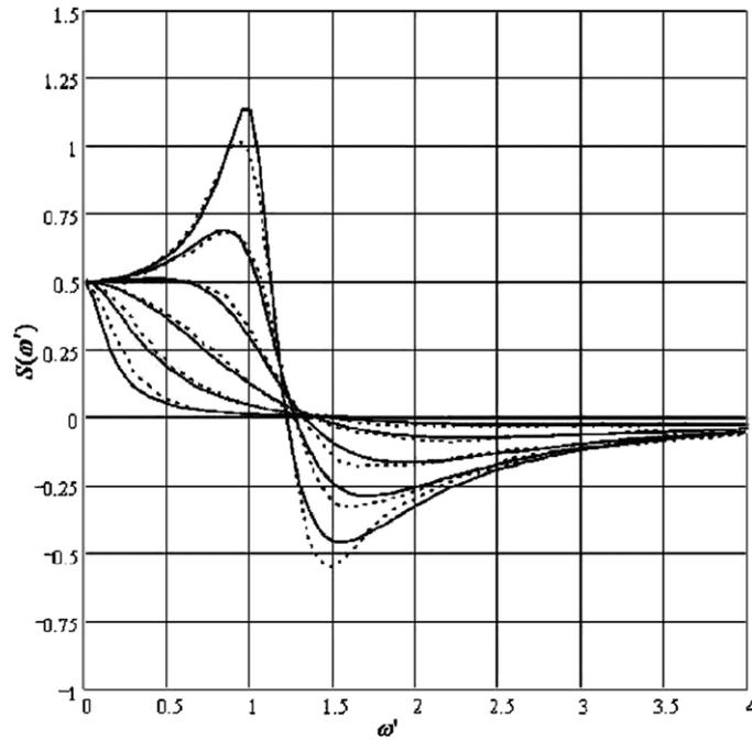
**Figure 6.** Normalized frequency shift for a constant velocity as a function of normalized applied frequency  $\omega' = \omega_0 R/v$ , for different values of the damping parameter  $r_o = R/\lambda$ . Solid curves: results of the analytic function, [50], equations (43) and (44). Dotted lines: numerical simulations from [50]. Starting at highest peak,  $r_o = 0.2, 0.5, 2, 4, 10$  (cylindrical cell).
