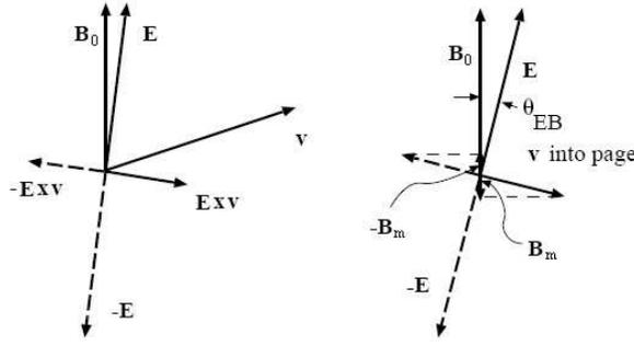
**Figure 2.** Geometrical picture of the  $\vec{E} \times \vec{v}$  effective magnetic field, where  $-B_m$  is indicated in the figure.
