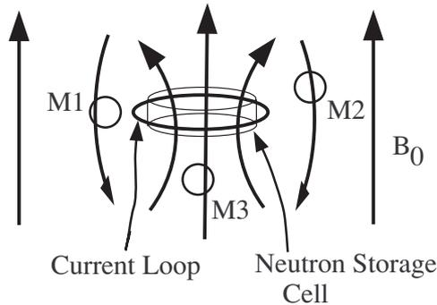
**Figure 4.** The external magnetometer problem. Leakage currents associated with the application of a high voltage to the measurement cell can flow in a loop (or some fraction thereof) around the cell, creating a magnetic field that is correlated with the direction of the electric field. Depending on the location of a magnetometer, the field from the loop can add or subtract to the applied static field  $B_0$ .
