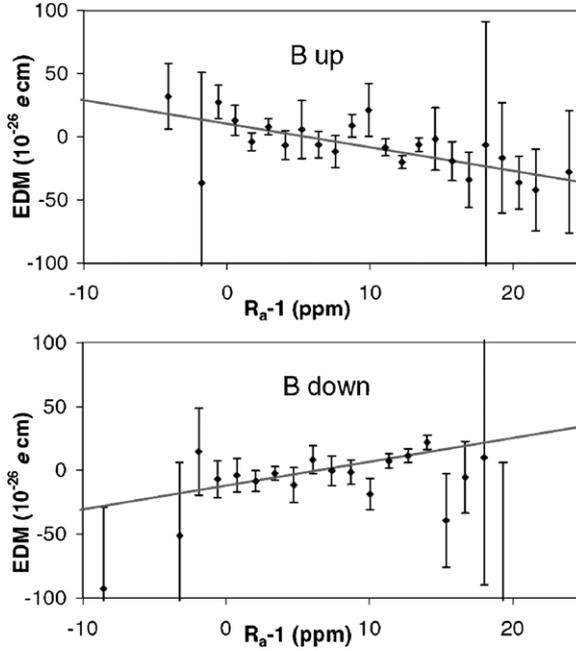
Figure 5. Apparent neutron EDM versus UCN-Hg frequency deviation from [48].
