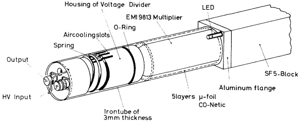
Fig. 2. Schematic drawing of a counter module.
