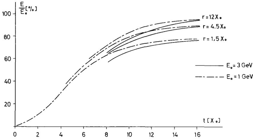
Fig. 1. The percentage of primary energy which is absorbed in a lead cylinder of radius  $r$  and length  $t$  (ref. 3).
