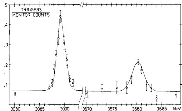
Fig. 1. Events with more than three tracks as counted by the trigger logic versus total energy of the two beams.
